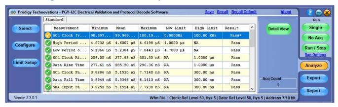
PGY-I2C runs inside the Tektronix oscilloscopes and makes the electrical measurements, decodes protocols and displays the decoded data in a bus diagram, a table, and links the decoded data to electrical signal in the bus diagram. I2C Protocol-based trigger can be setup using the built-in I2C trigger capabilities in Tektronix oscilloscopes.
